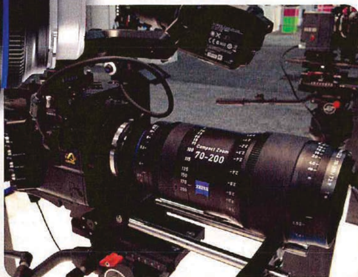
LEFT AND BELOW: The Zeiss CZ.2 15-30mm and 70-200mm zooms are both T2.9 and positioned to be companions to Ultra Prime lenses. BOTTOM: The Angénieux Optimo DP 25-250mm has a 10x zoom range and weighs only 16 pounds.
