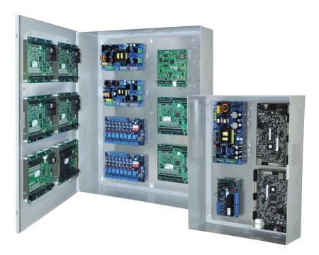
Trove<sup>™</sup> enclosures let installers easily combine Altronix power with myriad manufacturers' controllers and accessory boards. A host of backplanes are available supporting a wide range of options for scalable applications. Our solution allows you to easily configure and pretest power with various access control products prior to on-site installation.
